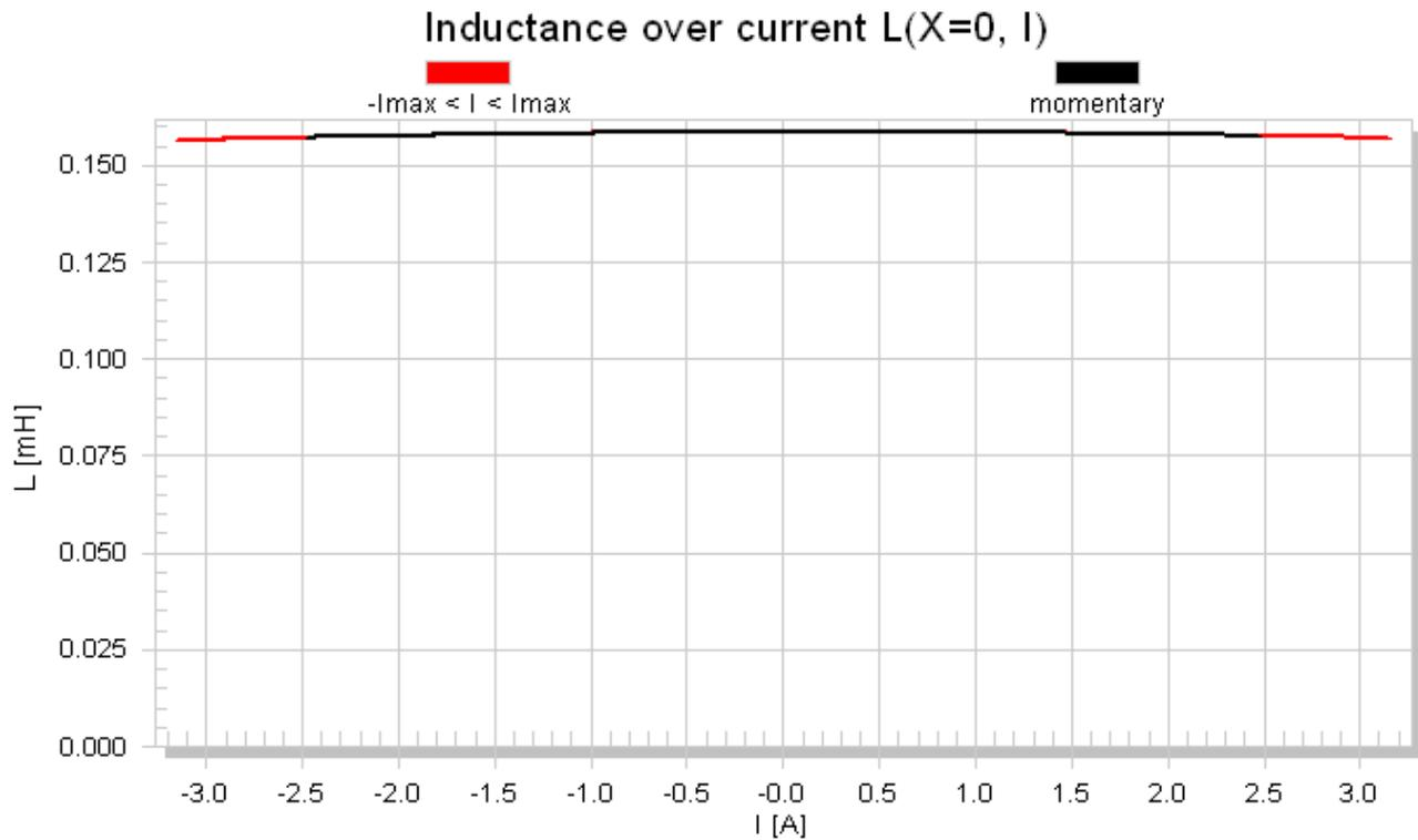
The inductance components  $L_e(x)$  and  $Bl(i)$  of most drivers have a strong asymmetric characteristic. If the voice coil moves towards the back plate the inductance usually increases since the magnetic field generated by the current in the voice coil has a lower magnetic resistance due to the shorter air path.
