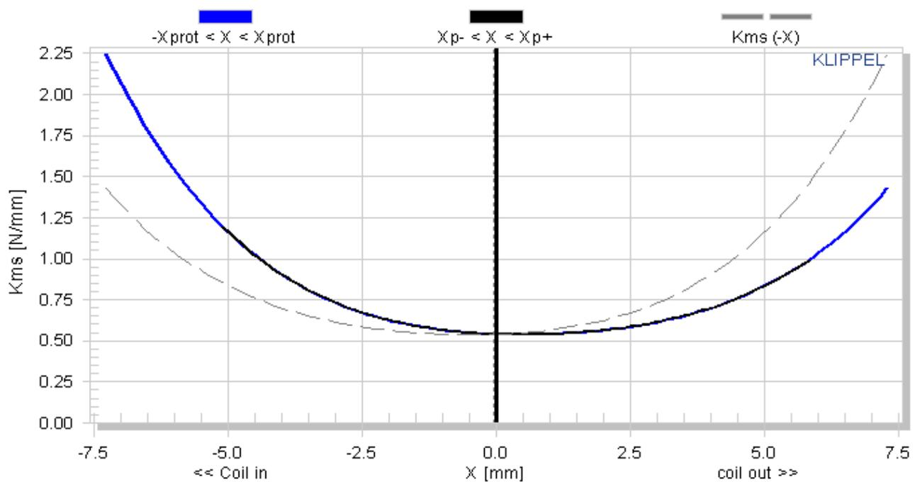
The stiffness  $K_{MS}(x)$  describes the mechanical properties of the suspension. Its inverse is the compliance  $CMS(x)$
