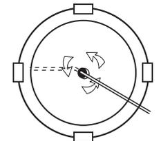
**CAUTION: Do Not Over-Tighten the Clamps. Too much torque may snap off the lug and the speaker will not seat securely. A snug fit is all that is necessary to assure proper performance.**
