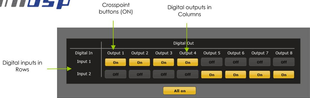
Note how labels of input channels and output channels followed on the Matrix mixer to simplify your routing. Let's illustrate the concept of configuration of this block using a 3way configuration + 2 subs where both Left & Right signals are being mixed (combined).
