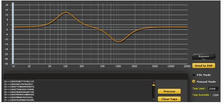
**Up to 10240 taps @ 48k / 4096 @96k** freely assignable in 8 sections of up to 2048 taps
